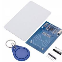
Gambar 2. RFID Module Mifare RC522
