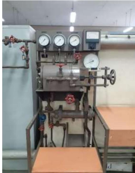
Gambar 1 Nozzle Rig Pada Steam Bench
