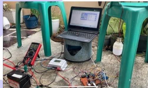
Gambar 7 Kondisi Relay Beban SoC 28% Lampu Padam
