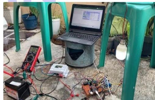
Gambar 8 Kondisi Relay Beban SoC 31% Lampu Nyala
