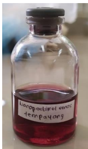
Figure 1. Result of Synthesis of Gold Nanoparticles with Malva Nut Gum Reducing Agent
