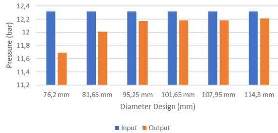
**Figure 7.** Comparison of Feed Tube Input and Output Pressure Parameters Based on ANSYS Fluent Validation
