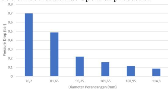
**Figure 4.** Pressure Drop Feed Tube Profile Based on Iteration Method
