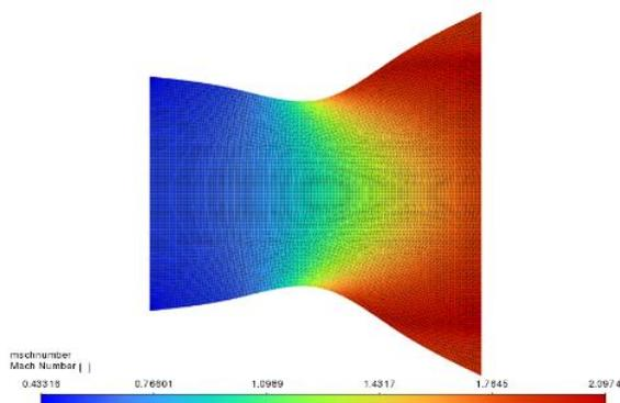
**Figure 12** Nozzle Simulation Results with Mach Number Parameters
