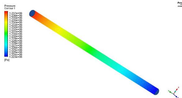
**Figure 8.** Fluid Computation Profile for Pressure Parameters on Feed Tube Diameter 101.65 mm
