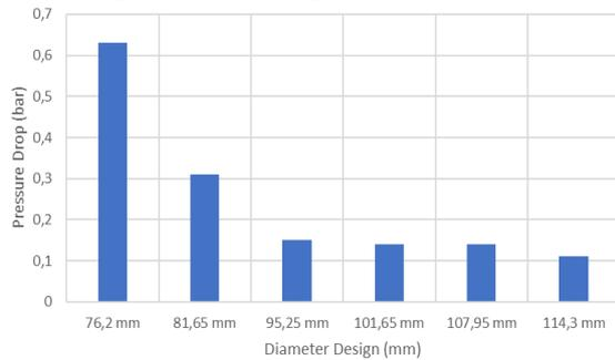
**Figure 9.** Pressure Drop Lance Tube Based on Iteration Method
