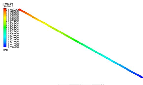
**Figure 11.** Fluid Computation Profile For Pressure Parameters On Lance Tube Diameter 114.6 mm
