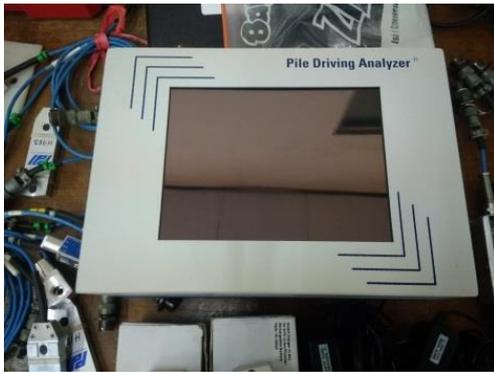
Gambar 10. Alat *Pile Driving Analyzer Test*
