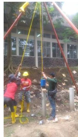
Gambar 9. Pengujian *Pile Driving Analyzer Test*
