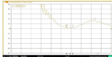
Gambar 13. Kurva SWR Antena Mikrostrip Artifisial  $TM_{01}$
