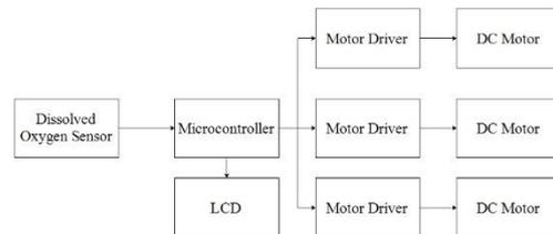
Figure 3 . 2 Block Diagram System
