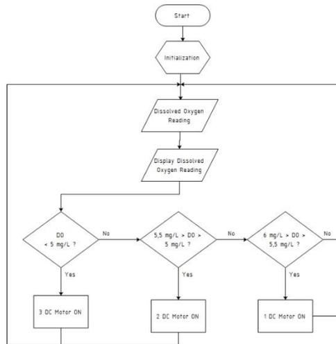
Figure 3. 3 Microcontroller Program Flowchart
