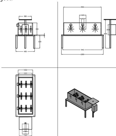
Figure 3. 4 Mechanical Design
