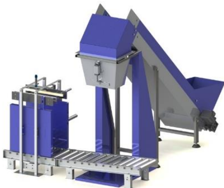
Gambar 8. 3D Model Mesin Pengemasan Silase
