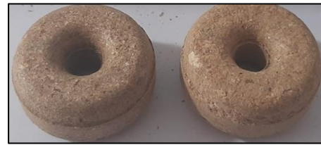
Gambar 10. Purwarupa briket limbah baglog jamur tiram
