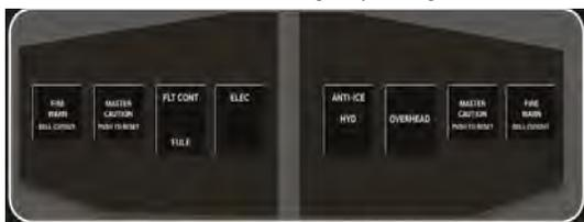
Gambar 14. Design of Master Fire Warning Light
