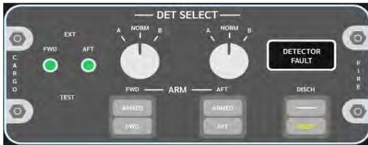
Gambar 13. Design of Cargo Fire
