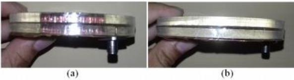
Gambar 8. Tampak samping (a) antenna mikrostrip artifisial; (b) antenna mikrostrip konvensional
