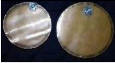
Gambar 7. Tampak belakang (a) antenna mikrostrip artifisial; (b) antenna mikrostrip konvensional
