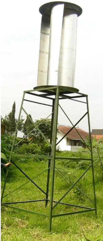
Gambar 11. Hasil assembling turbin angin
