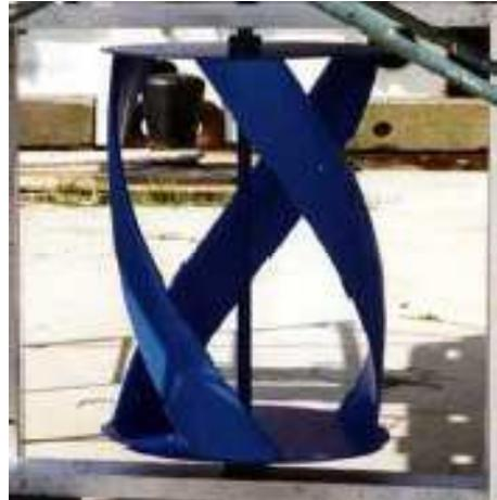
Gambar 1. Gorlov Helical Turbine (GHT) [4]
