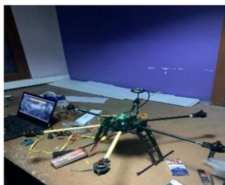
Gambar 3. Proses kalibrasi hexacopter
