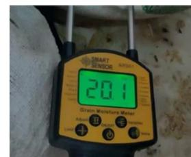
Gambar 15. Grain Moisture Sensor
