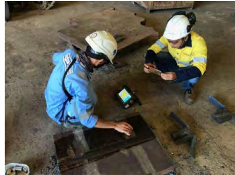
Gambar 17: Hasil Pengujian UT *Surface outside*
