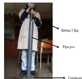
Gambar 2. Proses *repetitive hammering*
