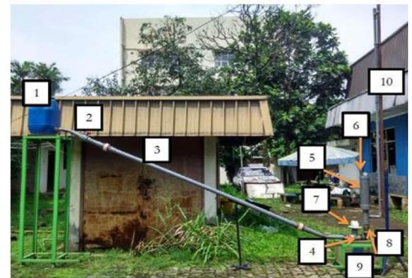
Gambar 7. Instalasi Pompa Hidram
