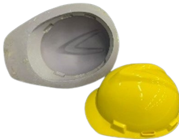
Gambar 4. Hasil manufaktur molding
