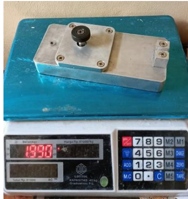
Gambar 9. Pengukuran Berat Special Tools Spherical Bearing Play Check
