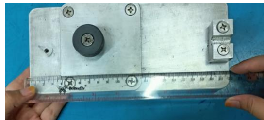
Gambar 7. Pengukuran Panjang Spherical Bearing Play Check
