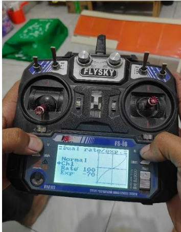
Gambar 7. Proses Pengkalibrasian motor servo
