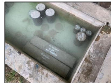
Gambar 5 Proses Perawatan ( Curing ) Beton
