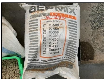
Gambar 3 Beton Instan K-275
