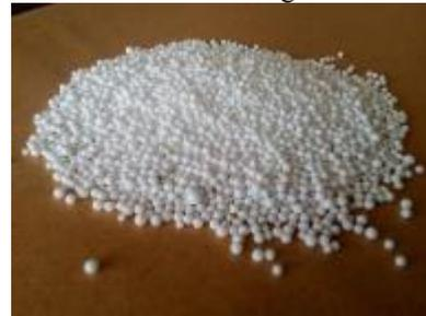
Gambar 9. Sampel EPS diameter SS
