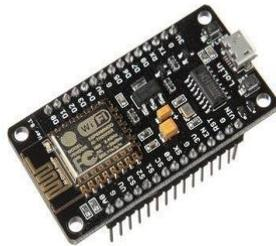
Gambar 4 NodeMCU
