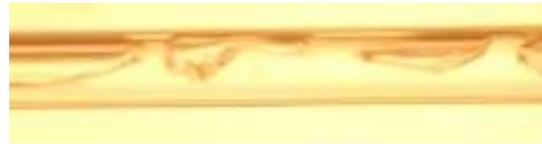
Gambar 3c: *Slug flow* pada pipa horizontal ( $J_L=0.012$  m/s,  $J_G=2.64$  m/s)
