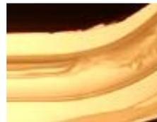
Gambar 4c: *Slug flow* pada pipa belokan ( $J_L=0.012$  m/s,  $J_G=2.64$  m/s)
