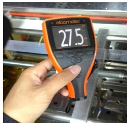
Gambar 2. Pengukur ketebalan (*thickness gauge*)
